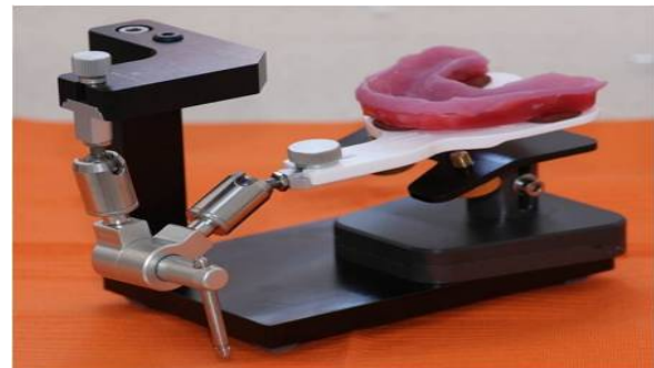
Fig. 4. Mounting the fork on the transfer table
