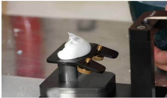
Fig. 5. Deposition of gypsum
